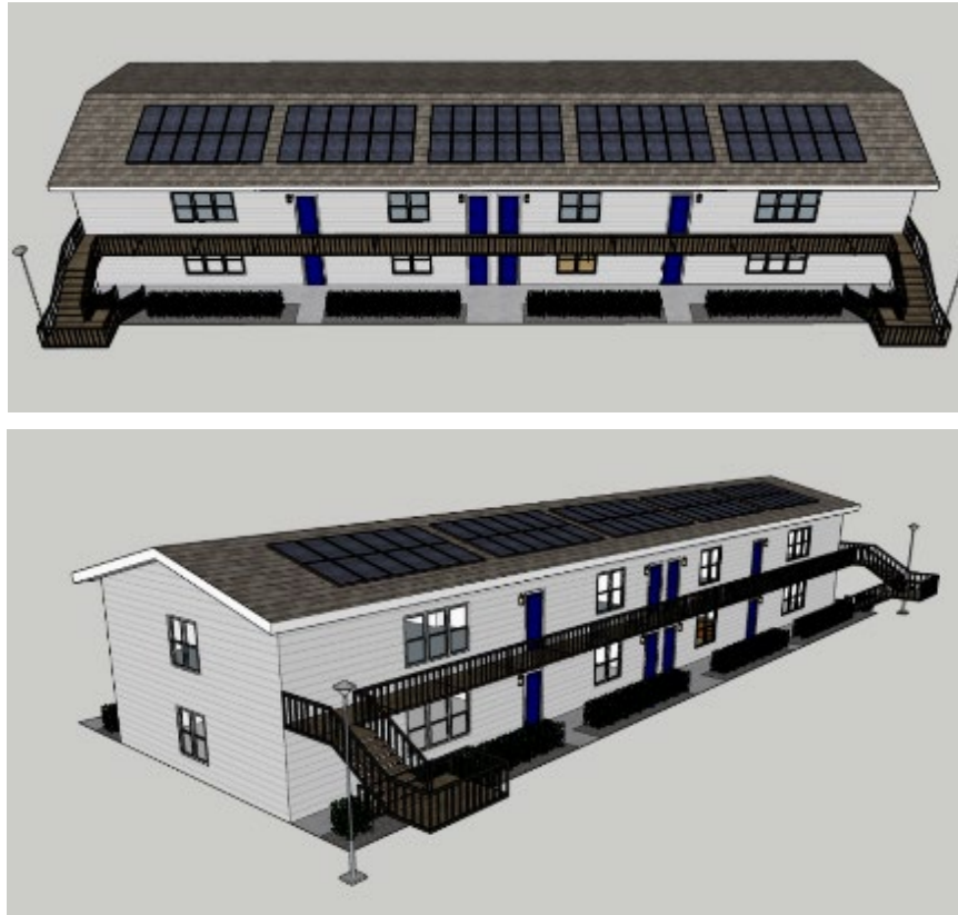
Figure 80: Garden Style Multifamily Case Study: Photovoltaics (PV) on South-Facing Roof
