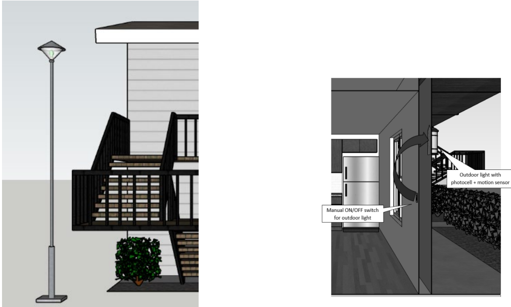
Figure 77: Garden Style Multifamily CASE Example: Outdoor Luminaires located on site (left); Dwelling Unit Entry Light and the entry switch on/off switch located inside the unit (right)
