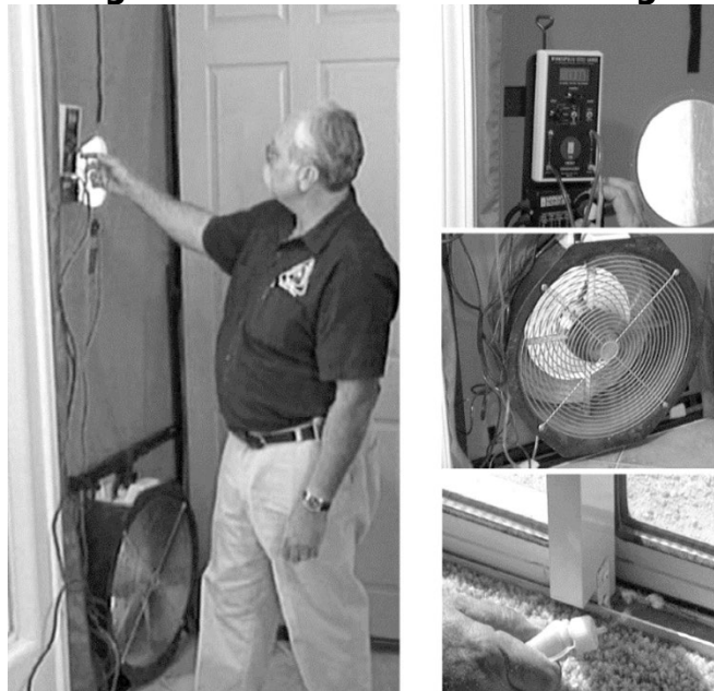
Figure 3-52: Blower Door Testing
