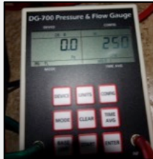
Duct Leakage to the Outside
