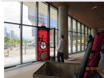
WHOLE BUILDING LEAKAGE REQUIREMENTS & RESULTS [leakage est. cubic feet per minute (CFM) per square foot at 50.00 Pascal]
