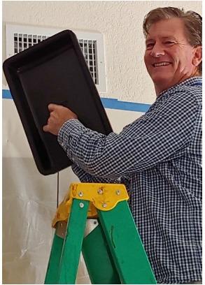
Duct Leakage Testing Equipment: Calibrated Fan Flowmeter
