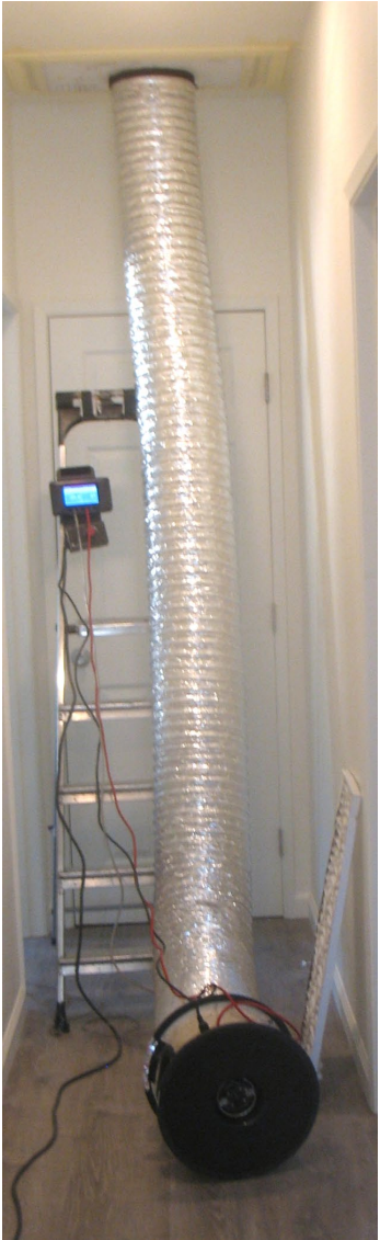
Duct Leakage Testing Equipment: Calibrated Fan Flowmeter
